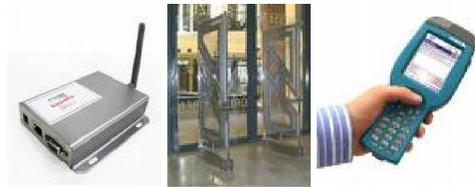
Fig. 3. Examples of RFID Readers
